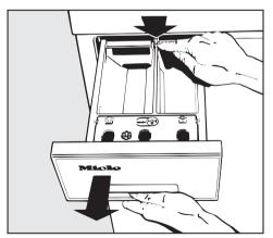
Pull out the detergent drawer until it stops. Press the red release lever down and pull the drawer out of the machine
